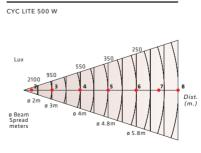
CYC LITE 500W - Model 53-70 L 242mm (9.53") 300mm (11.8") 105mm (4.13") KG 2.8kg (6.17 Lbs) 280x350x150mm (10.24"x13.78"x5.9")
